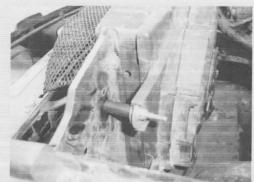
I tightened the assembly down with self-locking nuts and compressed the plastic housing against the metal frame of the radiator just tight enough to ensure it did not vibrate or rub.
