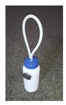
of brake fluid. Pump brakes and new fluid will fill system without back up due to built in check valve. Close bleed screw when finished, attach line back onto vent plug. No mess and easy! High qualty components.
