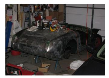
The paint was totally stripped, and any surface rust taken off, then treated and encapsulated just for extra insurance. I used epoxy primer and filled and sanded and filled and sanded............. My garage is still tinted blue
