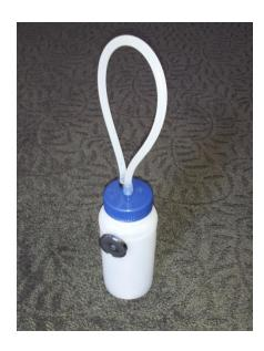
Try the One Man bleeder bottle the next time you need to replace brake fluid or after brake work to expel all air bubbles in the closed system.
