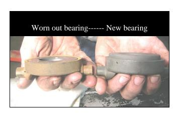
the clutch pedal where even the slightest pressure will push the throw out bearing against the clutch causing it to wear out prematurely.
