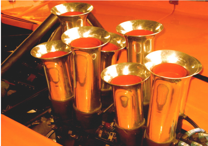
Can-Am McLaren intake stacks Photo by John Ulrich
